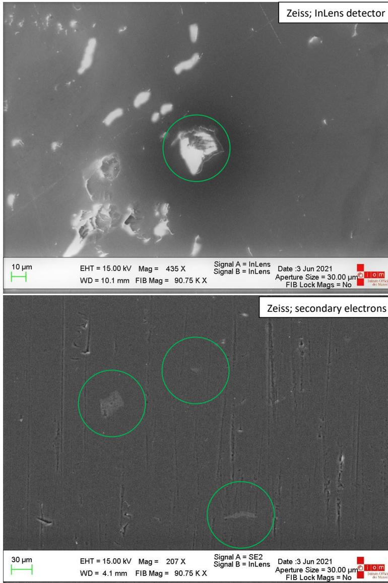
Figure 19-20 SEM image of two defects («unclassified defect» sample). Defects are indicated by green circles.
