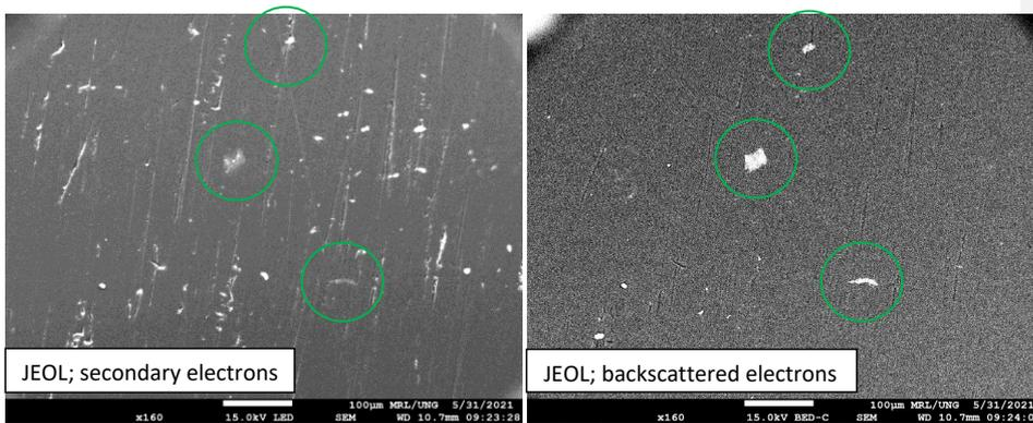
Figure 21 SEM image of the same defect imaged in fig.9, with secondary electrons (left) and backscattered electrons (right).
