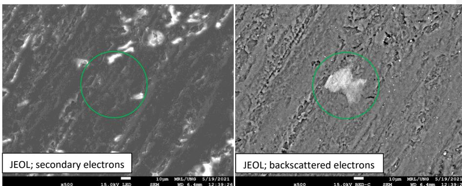
Figure 22 SEM image of the same area acquired with secondary electrons (left) and backscattered electrons (right).
