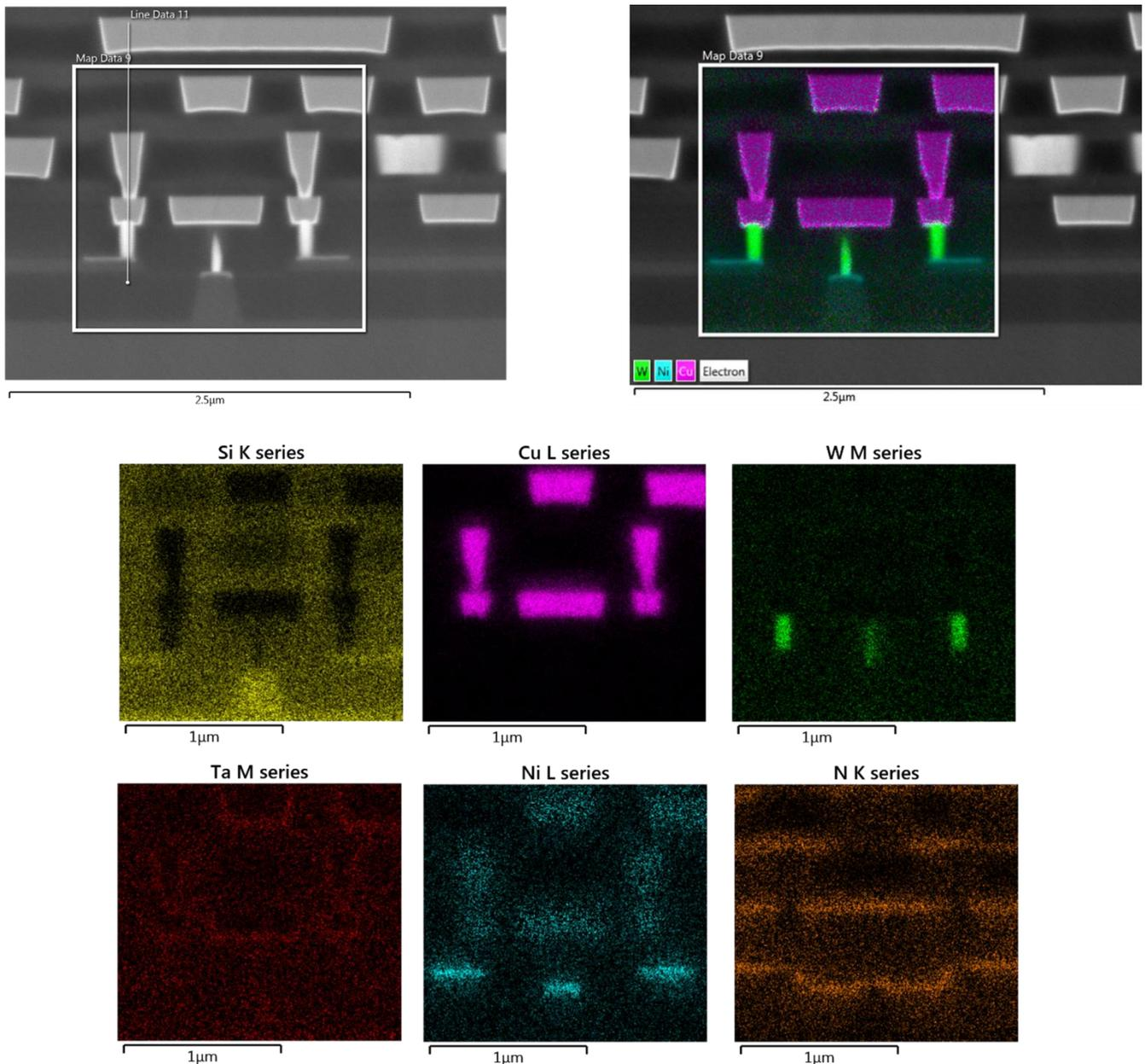
Figure 10: EDX elemental mapping at 5 KeV after point-by-point deconvolution of the EDX data
