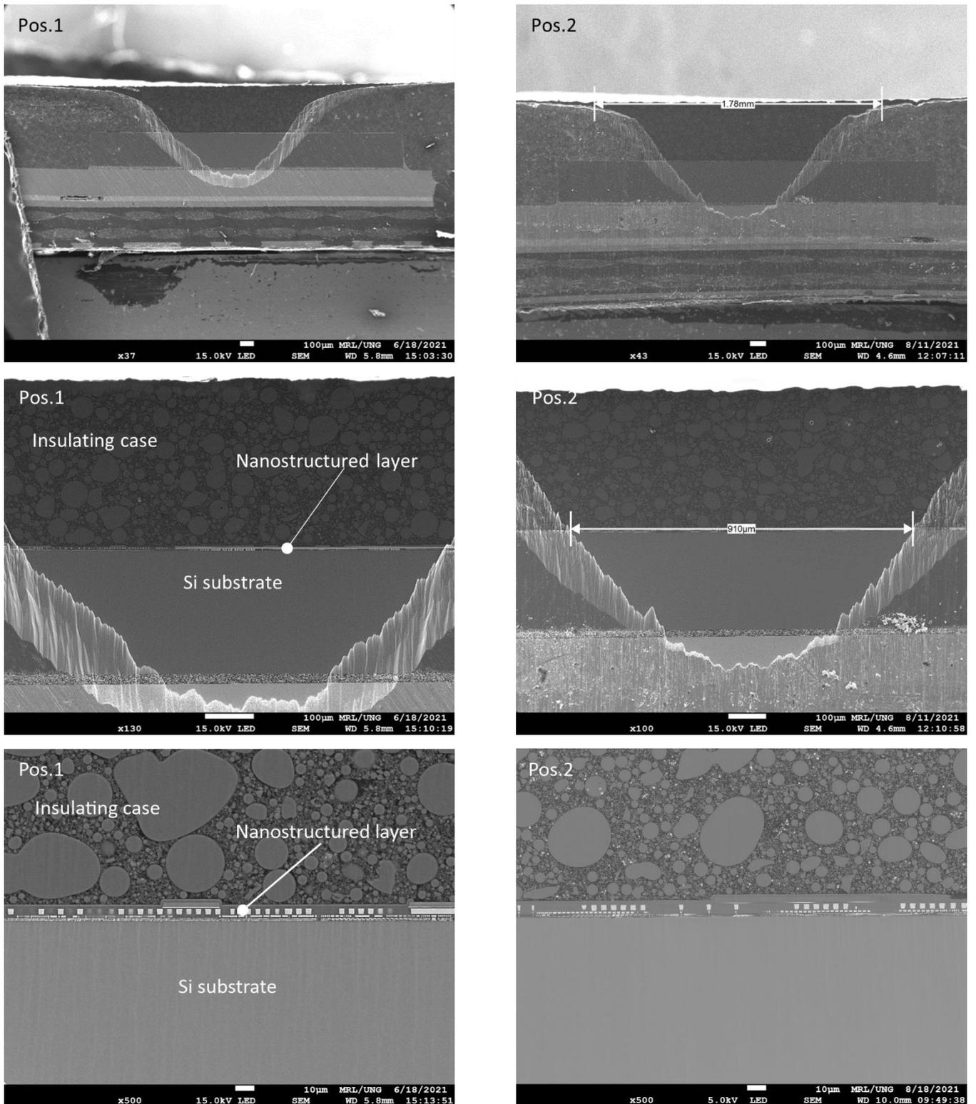
Figure 5: Low-mag SEM images of  $\text{Ar}^+$  ion polished cross sections at positions 1 and 2
