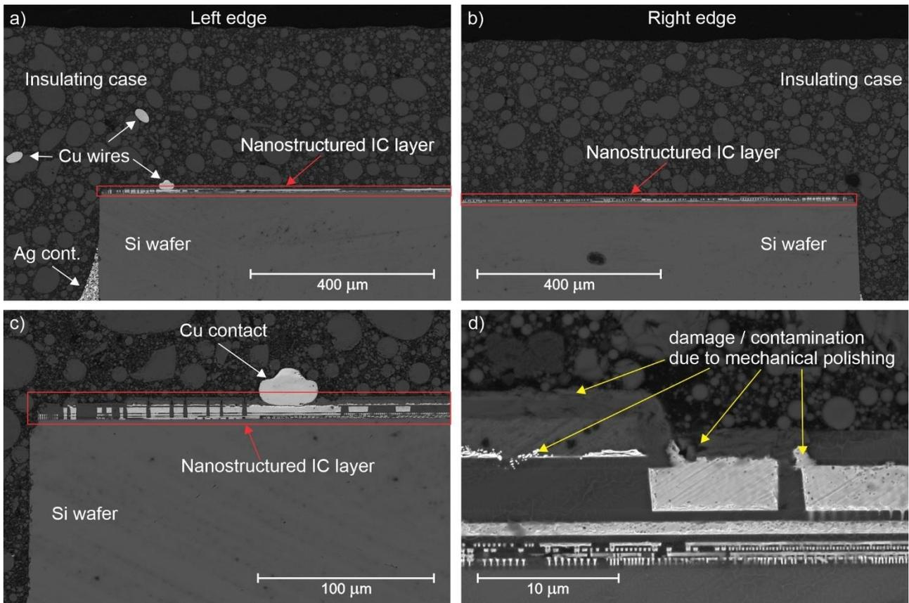
Figure 3: Phase contrast SEM images of mechanically polished IC component cross-section
