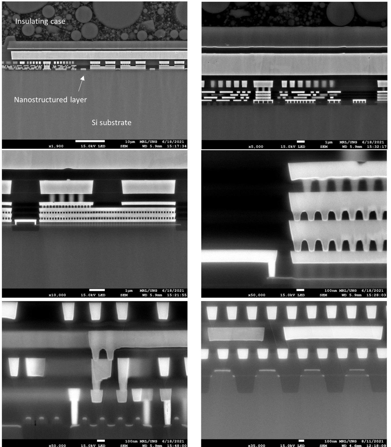
Figure 6: High magnification SEM images of Ar<sup>+</sup> ion polished cross sections of nanostructured IC layer
