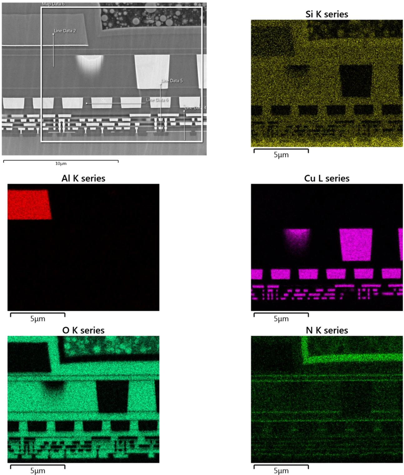
Figure 9: Typical set of EDX maps for major elements in nanostructured IC layer
