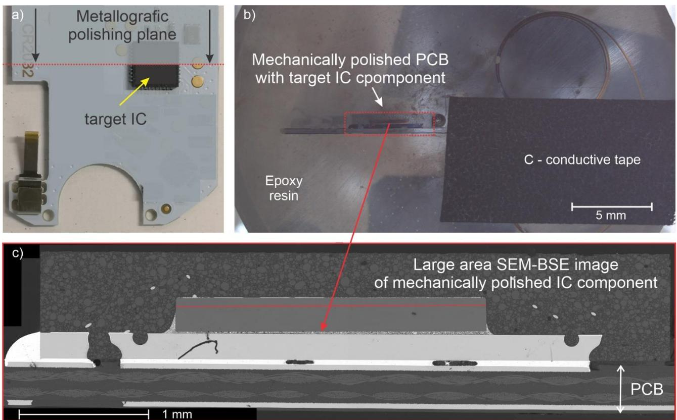
Figure 1: Position of mechanically polished electronic device (a) with optical image of freshly exposed cross-section - target IC component on top of PCB (b) and corresponding large area SEM-BSE image (c)
