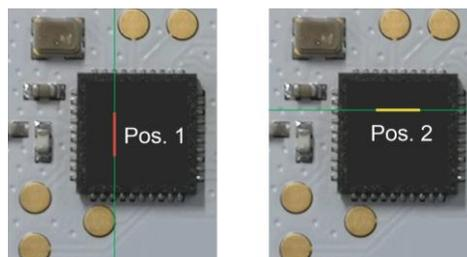
Figure 4: Locations of Ar<sup>+</sup> ion polished cross sections on the IC
