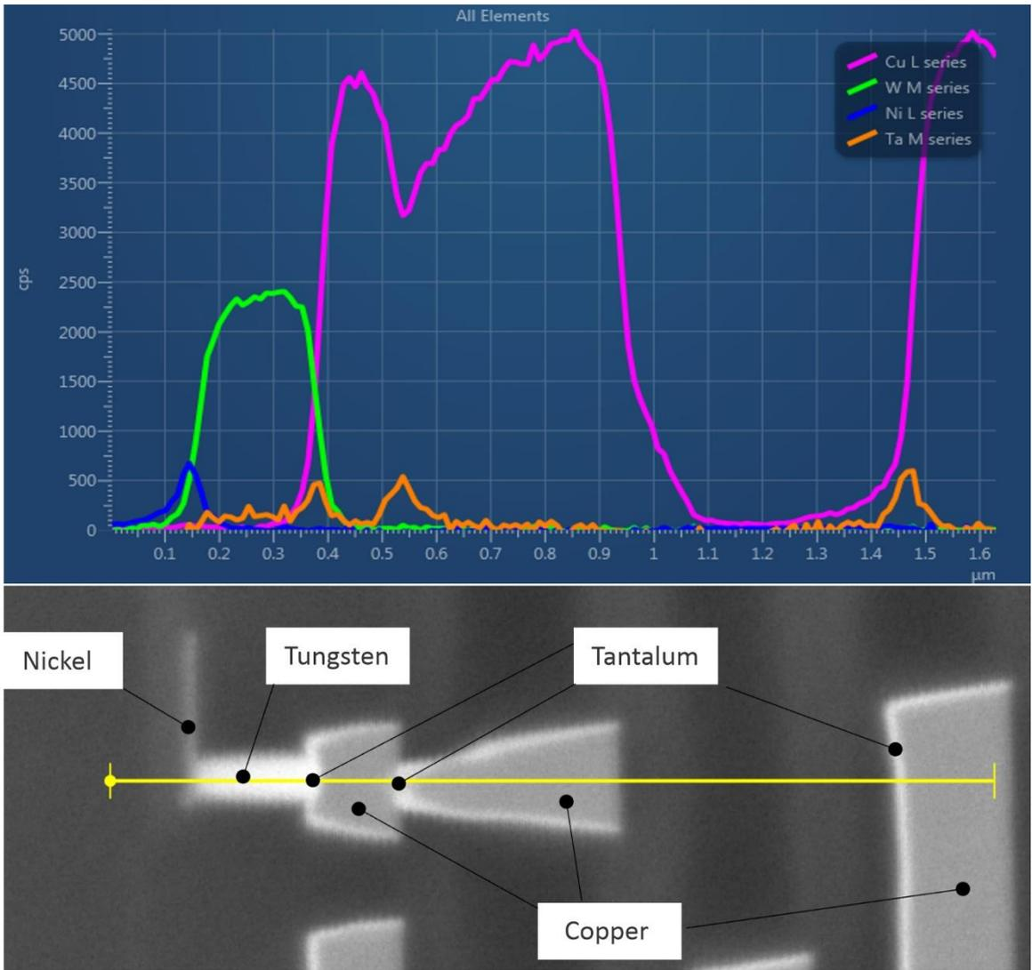
Figure 11: EDX Linescan profiling at 5 KeV after deconvolution of the EDX data
