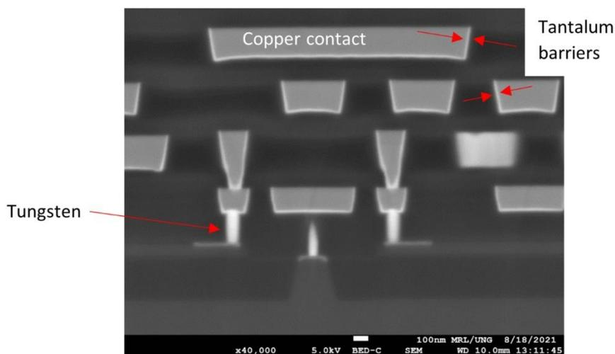
Figure 8: High magnification SEM images of Ar<sup>+</sup> ion polished cross sections of nanostructured IC layer
