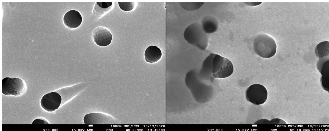
Figure 6: Scanning electron microscopy of Au coated membrane (left) before and (after) particle deposition.
