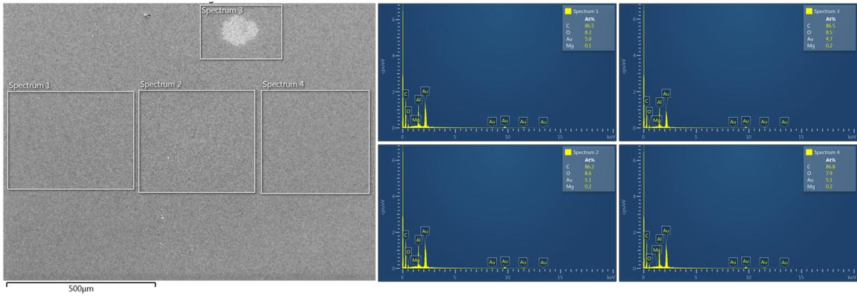
Figure 7: EDX based analysis of Au coated membrane before particle deposition. Analysed region corresponds to area presented in Figure 3.
