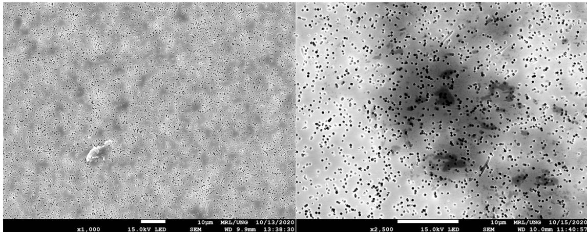
Figure 4: Scanning electron microscopy of Au coated membrane (left) before and (right) after particle deposition.
