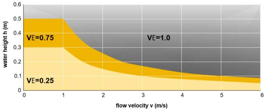
Figure S6: Vulnerability values as a function of the water height ( $h$ ) and the flow velocity ( $v$ ) for: (a) vineyards, (b) orchard and olive trees, (c) vegetables, and (d) natural and semi-natural environments, derived from laboratory experiments (Citeau, 2003)
