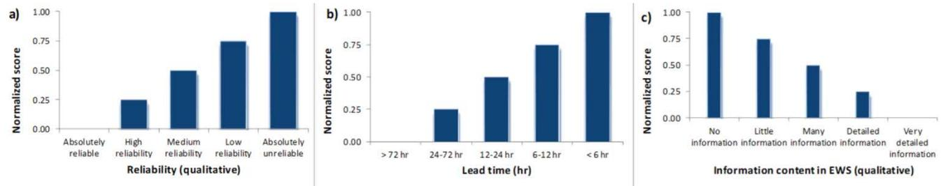
Figure S3: Value functions for the vulnerability indicators that are part of evaluating the Adaptive Capacity (De Luca, 2013)
