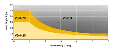
Figure S6: Vulnerability values as a function of the water height (h) and the flow velocity ( $\nu$ ) for: (a) vineyards, (b) orchard and olive trees, (c) vegetables, and (d) natural and semi-natural environments, derived from laboratory experiments(Citeau, 2003)
