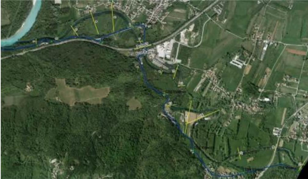
Figure 3: Cross sections measured by FVG topographical survey on Italian side
