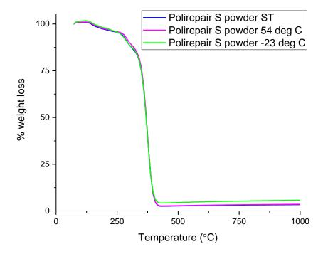
**Figure 1.** Thermogravimetric analysis of the Polirepair S powder samples.
