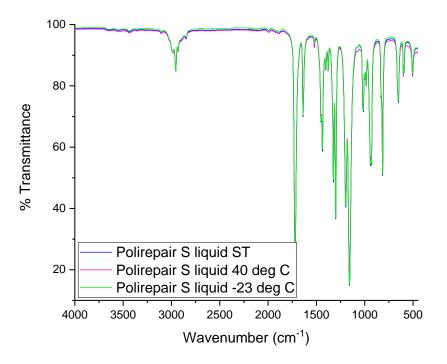
Figure 4. FT-IR spectrum of the Polirepair S liquid samples.
