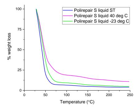
Figure 2. Thermogravimetric analysis of the Polirepair S liquid samples.
