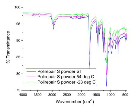
Figure 3. FT-IR spectrum of the solid Polirepair S powder samples.
