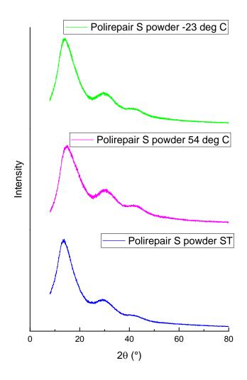
Figure 5. PXRD patterns of the solid Polirepair S samples.
