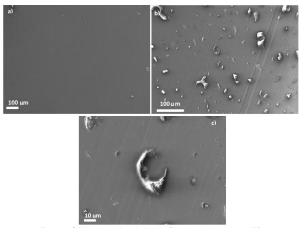
**Figure 7.** SEM images of the Polirepair S sample incubated at 60 °C.
