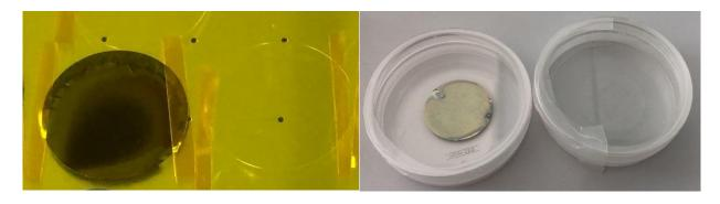
Figure 4 Slides, metallized or not, after functionalization and insertion into petri dishes
