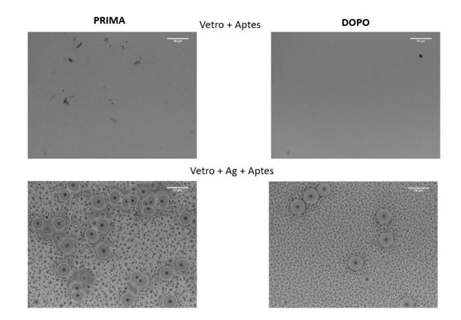
Figure 5 Optical microscopy images of the glass samples, with or without Ag metallization, functionalized with APTES, BEFORE and AFTER the sanitization process.
