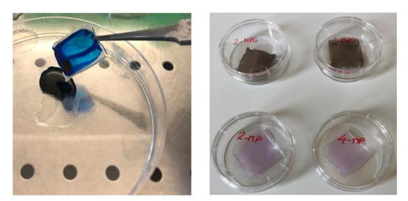
Figure 8. Left, a specimen subjected to Giemsa staining. On the right, the metallized (top) and non-metallized (bottom) samples after Giemsa staining.
