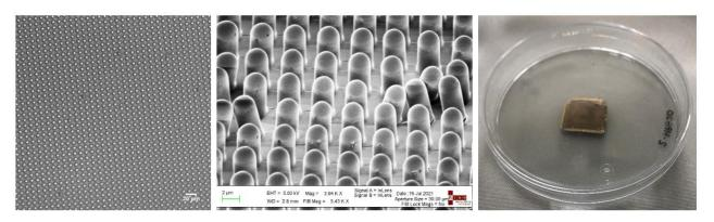
Figure 6 Image of the micro pillars acquired by optical and SEM microscopy, and the substrate of PDMS glued on a 92 mm Petri dish.
