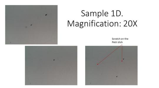
Figure 3 Examples of images acquired with an optical microscope. The particles present seem to be attributable to dirt or contamination not of bacterial origin.
