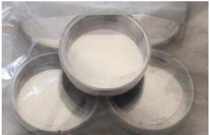
Figure 1 Example of plates metallized with Ti-Ag
