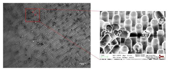
Figure 7 On the left, the optical microscopy image of the Au-coated micropillars on which structures morphologically similar to the bacterial ones were found. On the right, the SEM image that highlights how these structures were disjoint pillars.
