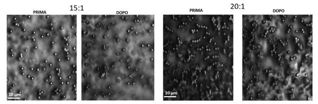
Figure 10. Images acquired under an optical microscope of the substrates with a ratio of 15: 1 (left) and 20: 1 (right) on which the company sampled, before and after the sanitization process.
