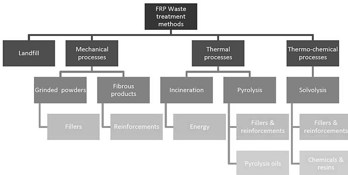
Figure 12: Schematic presentation of different FRP waste recycling technologies and processes (adopted from <http://www.windfarmbop.com>)
