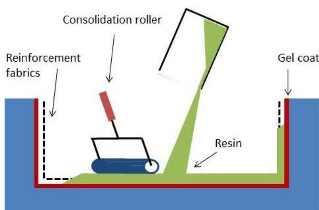
Figure 3: A simplified sketch of Hand lay-up forming process of FRP production (source: ZAG internal - documentation)
