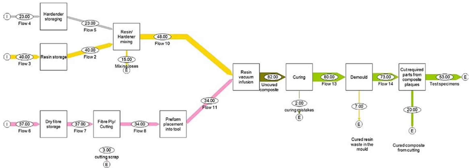
Figure 10: Example of material flow analysis in FRP production line (generated with STAN2 software); (I-Input, E-material output; adopted from Rybicka et al., 2015)
