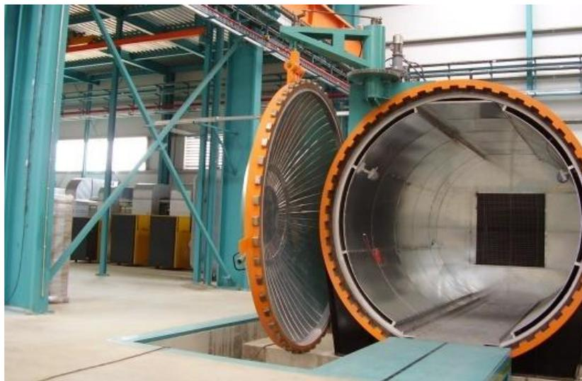
Figure 5: An example of autoclave moulding setup (source: JaviRD on Wikimedia Commons)
