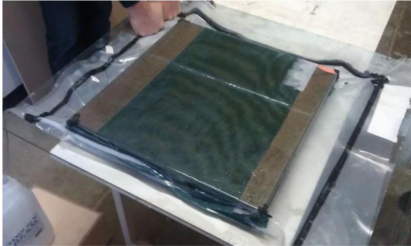
Figure 4: Preparation of simple FRP plate by vacuum bag moulding (source: ZAG internal photo-documentation)
