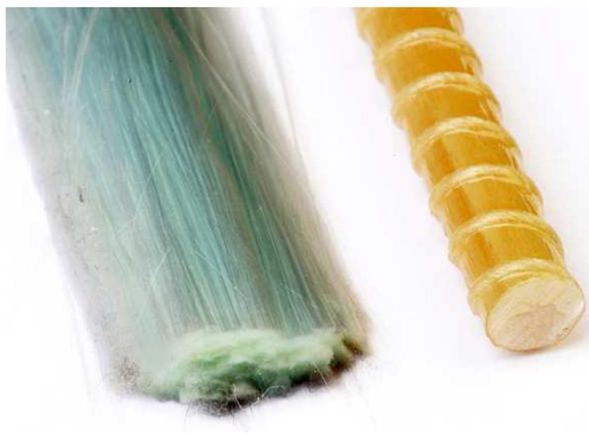
Figure 14: Fibres recovered by thermal degradation of FRP product (left) and reinforcement rod from such fibres (right).
