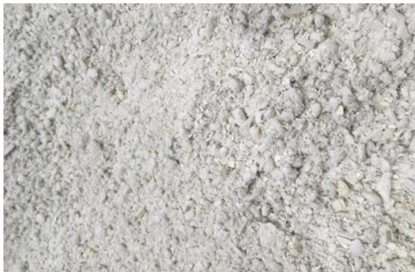
Figure 13: A mechanically processed FRP waste in a form of a fine granulate (internal photo documentation of ZAG)
