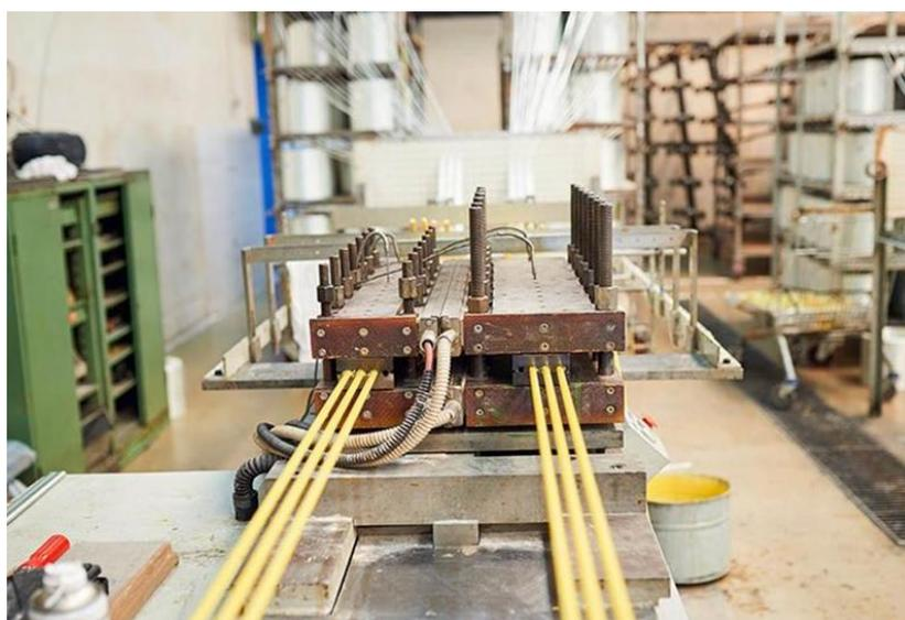
Figure 7: The photo of the finished FRP rods at the end of the pultrusion process (source: internal photo-documentation of the Trival Kompoziti d.o.o.)
