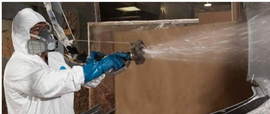
Figure 9: The lay-up of the glass fibre / resin mixture with the chopper gun (source: photo on [www.graco.com](http://www.graco.com))
