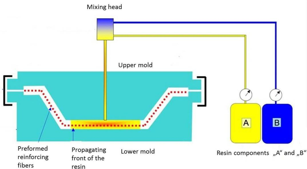
Figure 8: The scheme of production of FRP product with Resin Transfer Moulding (source: Laurens van Lieshout on Wikimedia Commons)
