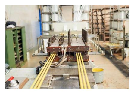
Figure 7: The photo of the finished FRP rods at the end of the pultrusion process (source: internal photodocumentation of the Trival Kompoziti d.o.o.)
