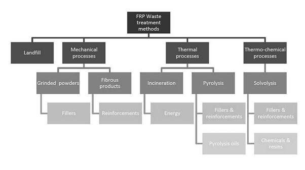
Figure 12: Schematic presentation of different FRP waste recycling technologies and processes (adopted from <a href="http://www.windfarmbop.com">http://www.windfarmbop.com</a>)
