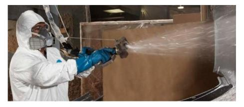
Figure 9: The lay-up of the glass fibre / resin mixture with the chopper gun (source: photo on www.graco.com)
