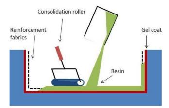
Figure 3: A simplified sketch of Hand lay-up forming process of FRP production (source: ZAG internal - documentation)
