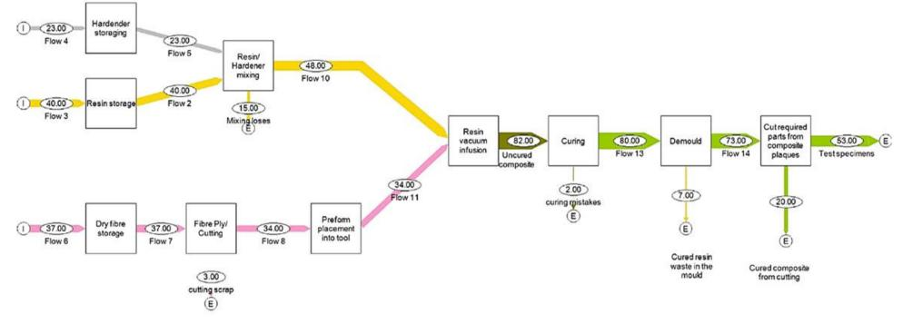
Figure 10: Example of material flow analysis in FRP production line (generated with STAN2 software); (I-Input, E-material output; adopted from Rybicka et al.,
