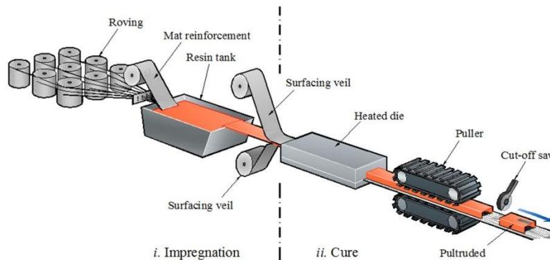
**Figure 6:** Schematic presentation of pultrusion process of FRC production (Source: Landesmann et al. 2015).
