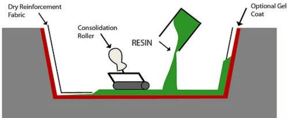
**Figure 2:** A simplified sketch of Hand lay-up forming process of FRC production (source: Vadivelvivek 2013)
