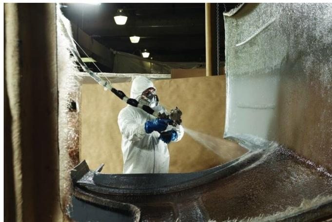
**Figure 7:** Example of Chopper gun lay-up process usually used for reinforcing of large FRC products, like vessels.
