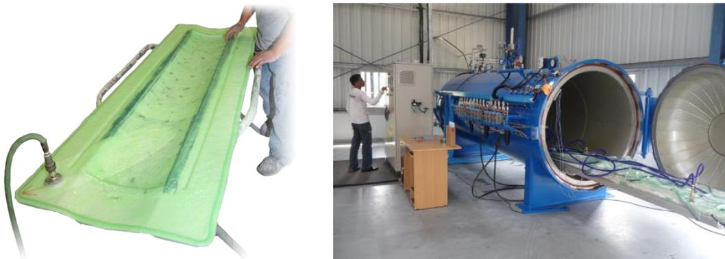
**Figure 3:** Types of FRC forming processes. Left: Vacuum bag moulding of FRC products (source: [www.reynoldsam.com](http://www.reynoldsam.com)). Right: An example of autoclave moulding (source: [www.reinforcedplastics.com](http://www.reinforcedplastics.com))
