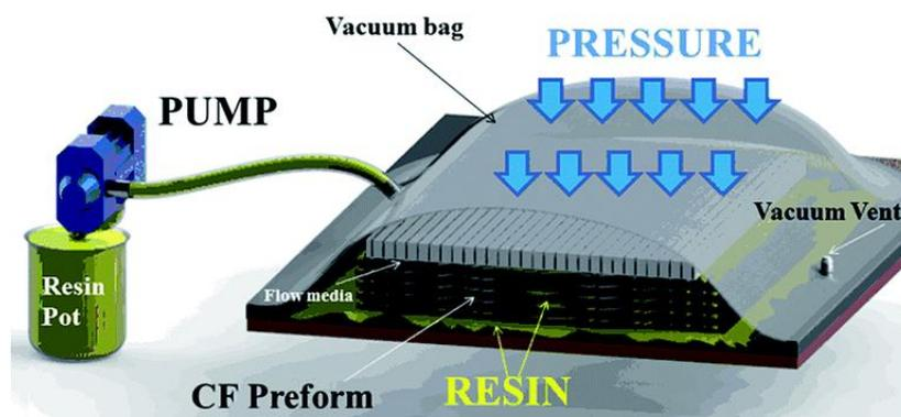
**Figure 5:** An example of resin infusion production of FRC (source: Guadagno et al. 2015)
