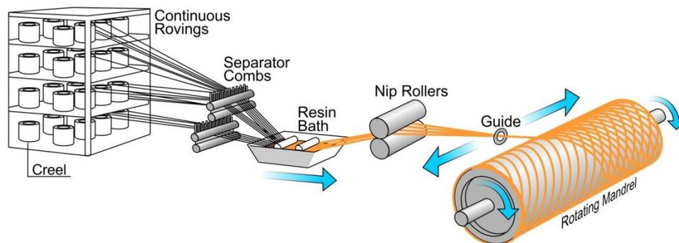
**Figure 4:** Schematic presentation of filament winding process in FRC production (Source: [www.nuplex.com](http://www.nuplex.com)).
