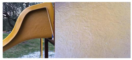
Figure 9: An example of FRC product. Left: Slide. Right: Detail view of the slide's back surface (Photo: A. Mauko Pranjić).
