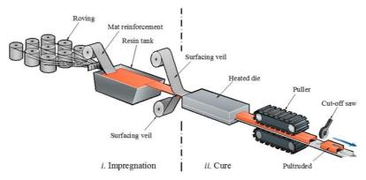
Figure 6: Schematic presentation of pultrusion process of FRC production (Source: Landesmann et al. 2015).
