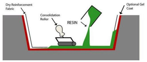
Figure 2: A simplified sketch of Hand lay-up forming process of FRC production (source: Vadivelvivek 2013)
