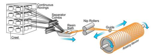
Figure 4: Schematic presentation of filament winding process in FRC production (Source: <u>www.nuplex.com</u>).
