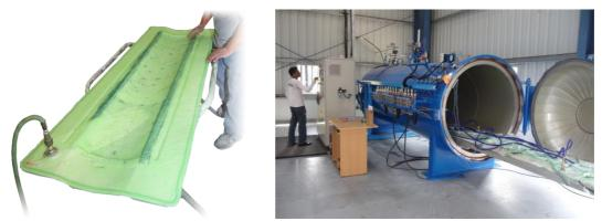
**Figure 3:** Types of FRC forming processes. Left: Vacuum bag moulding of FRC products (source: <u>www.reynoldsam.com</u>). Right: An example of autoclave moulding (source: <u>www.reinforcedplastics.com</u>)
