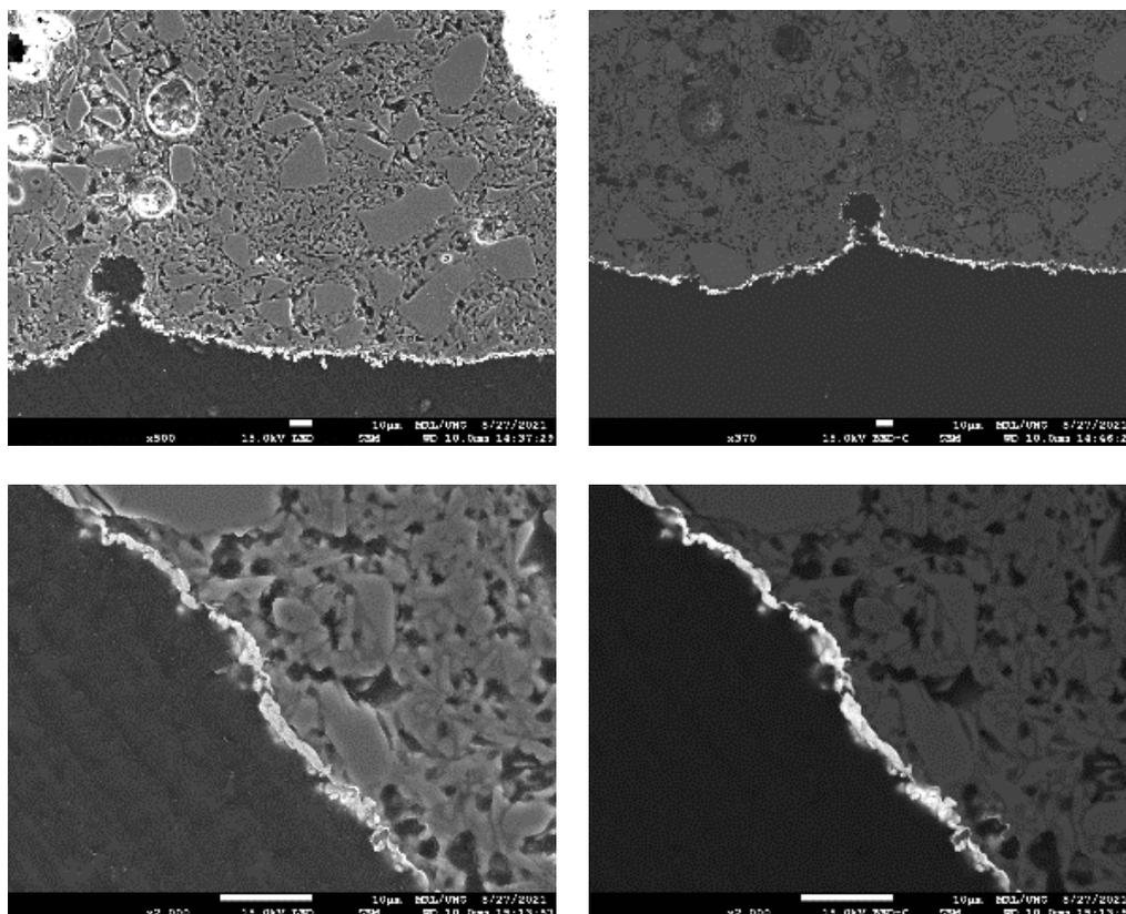
Figure 3: SEM images of W-coated SiC, after fracturing, embedding in epoxy resin, cutting and mechanical polishing (down to 3 µm diamond abrasive) observed by secondary electrons (left) and back scattered electrons (right).
