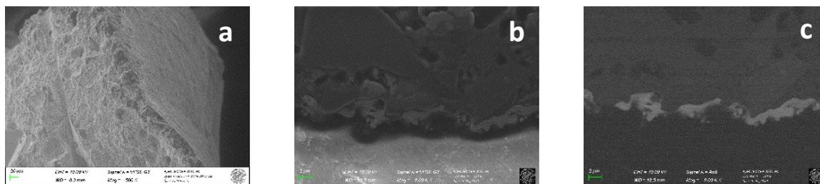
Figure 2: SEM images of bare porous SiC after fracturing (a) and W-coated SiC, after fracturing, embedding in epoxy resin, cutting and mechanical polishing (down to 3 µm diamond abrasive) observed by secondary electrons (b) and back scattered electrons (c).
