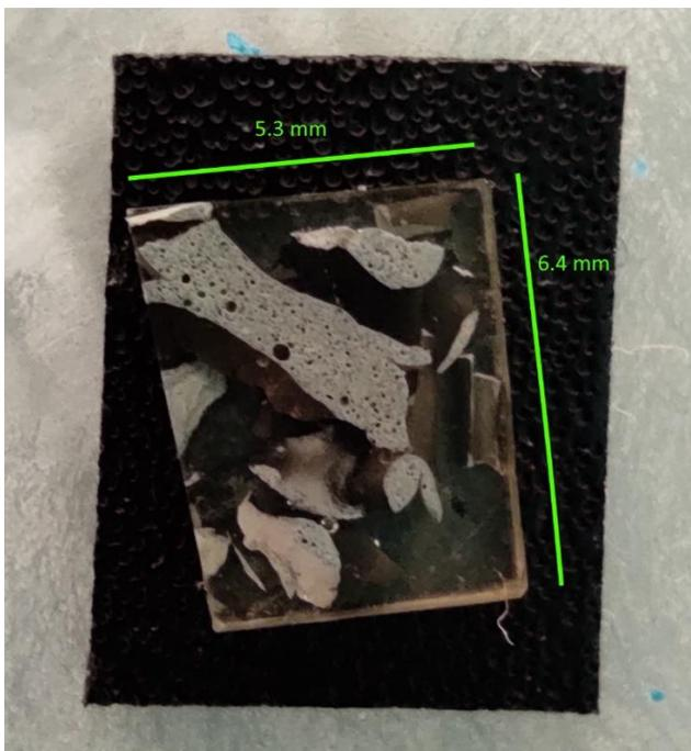
Figure 1: Picture of W-coated sample embedded in epoxy resin, after cutting and mechanical polishing.
