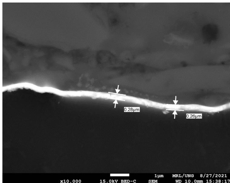
Figure 5: BSE images of W-coated SiC. The thickness of the W metallic layer in this region is  $(0.27 \pm 0.01) \mu\text{m}$ .
