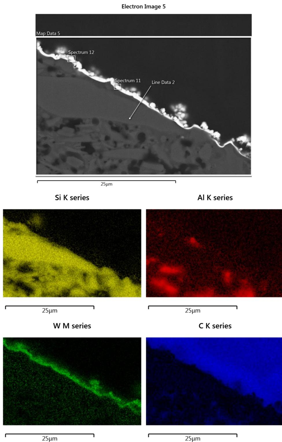
Figure 6: SEM (top) and EDX maps of Si, Al, W and C. Observation conditions: Imaging: beam energy 10-15 KeV; secondary electron detector. EDX mapping and spectroscopy: beam energy: 15 KeV.
