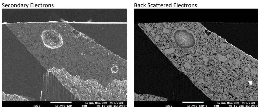
Figure 4: SEM images of W-coated SiC. after mechanical polishing and X-section Ar-ion polishing observed by secondary electrons (left) and back scattered electrons (right).
