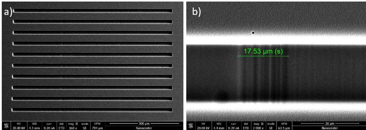
Fig 3. FIB analysis of stitches in sample 48S: a) line pattern with indicated stitches, b) 7000 x magnified image of single stitch in line pattern
