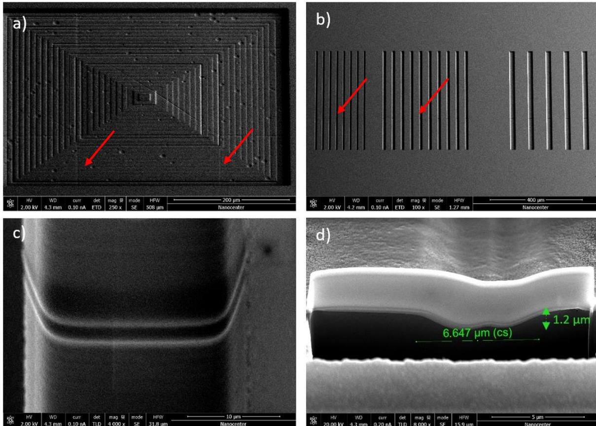
Fig 2. FIB analysis of stitches in sample 10S: a) pyramid pattern with indicated stitches, b) line pattern with indicated stitches, c) 4000 x magnified image of single stitch in line pattern, d) FIB cross-section across stitch with measurements of the width and depth of a stitch.
