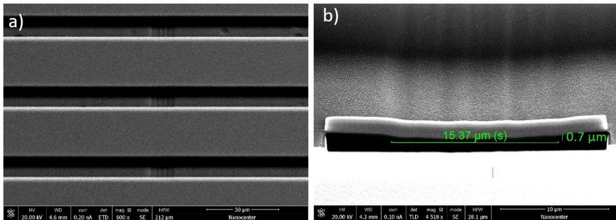
Fig 4. FIB analysis of stitches in sample 72S: a) line pattern with indicated stitches, b) FIB cross-section across stitch with measurements of the width and depth of a stitch.
