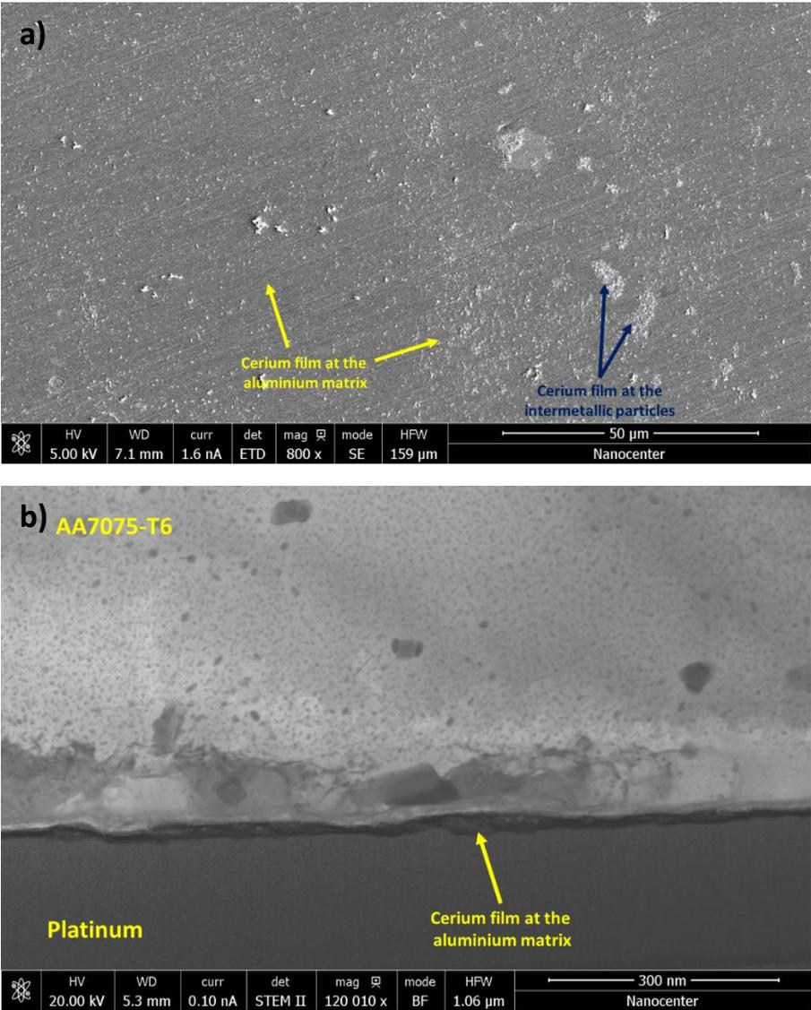
Figure 1: a) Surface appearance of AA7075-T6 immersed for 6 hours in NaCl + Ce(OAc)<sub>3</sub> solution, b) FIB cross-section of AA7075-T6 immersed for 6 hours in NaCl + Ce(OAc)<sub>3</sub> solution
