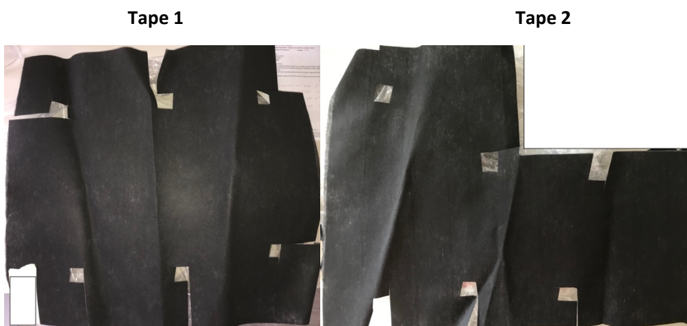
Figure 1: Photograph of two non-woven tapes of approximately 0.5m x 0.5m. Left tape was labeled Tape 1 and right tape was labeled Tape 2. Empty gaps represent missing pieces, which were further shaped and electrically characterized.
