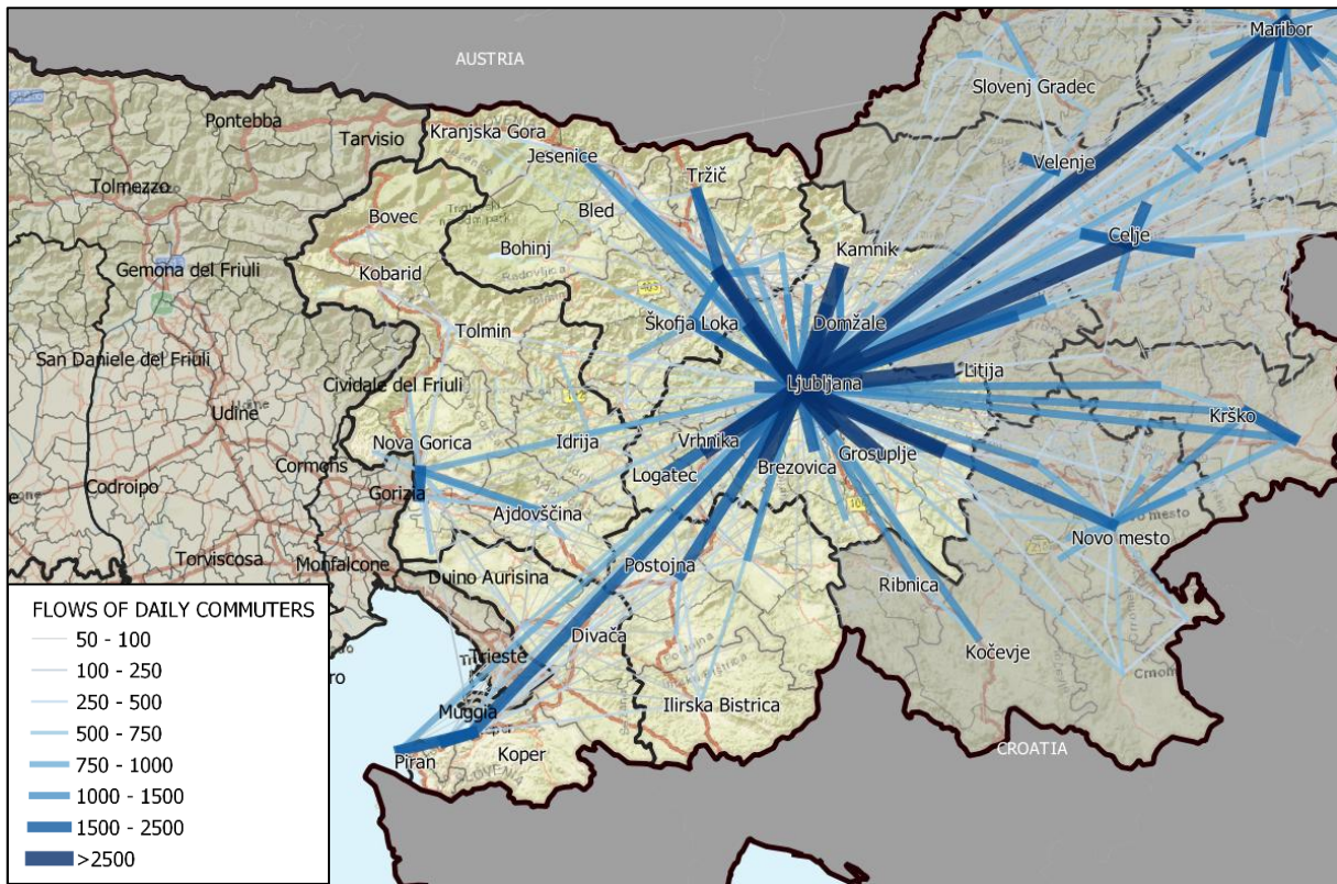
Figure 28 – Desire lines of related to commuters’ transport demand between Slovenian municipalities. Source: Elaborations on SURS data (SiStat database).
