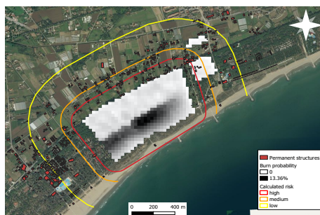
Basemap from Bing™ maps service ©Microsoft 2020. Fig. 2 Risk contours based on thermal effect on permanent light structures.
