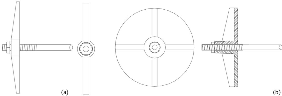
Fig. 69: Threaded ties: tie with end nut and holed anchor head (a); circular cast iron anchor (b)
