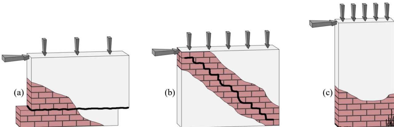
Fig. 12: Failure mechanism of masonry.
