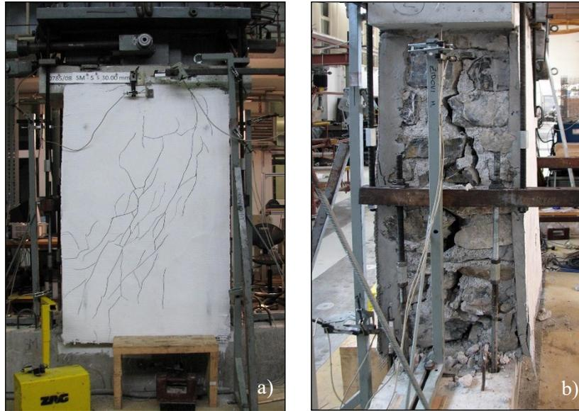
Fig. 53: Stone wall with coating on both sides during test. Shear damage on the coating (a), splitting of the wall due to lack of diatones (b).
