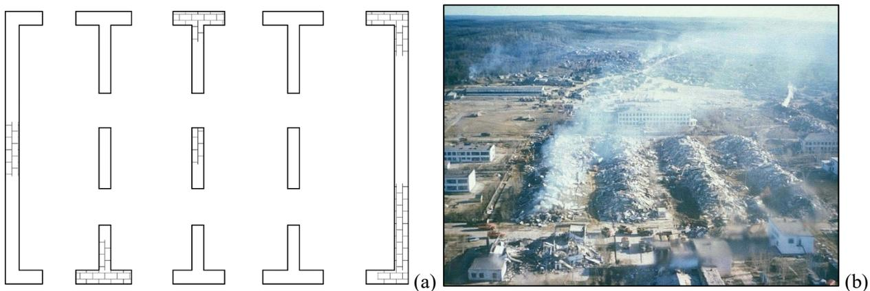
Fig. 10: a) uneven distribution of resisting elements in perpendicular directions, b) Collapse in one direction (Neftegorsk, Russia 1995)
