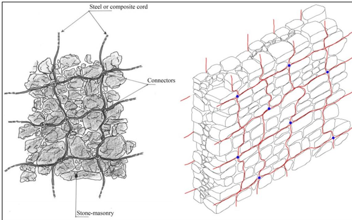
Fig. 62: Structural repointing with steel strands.
