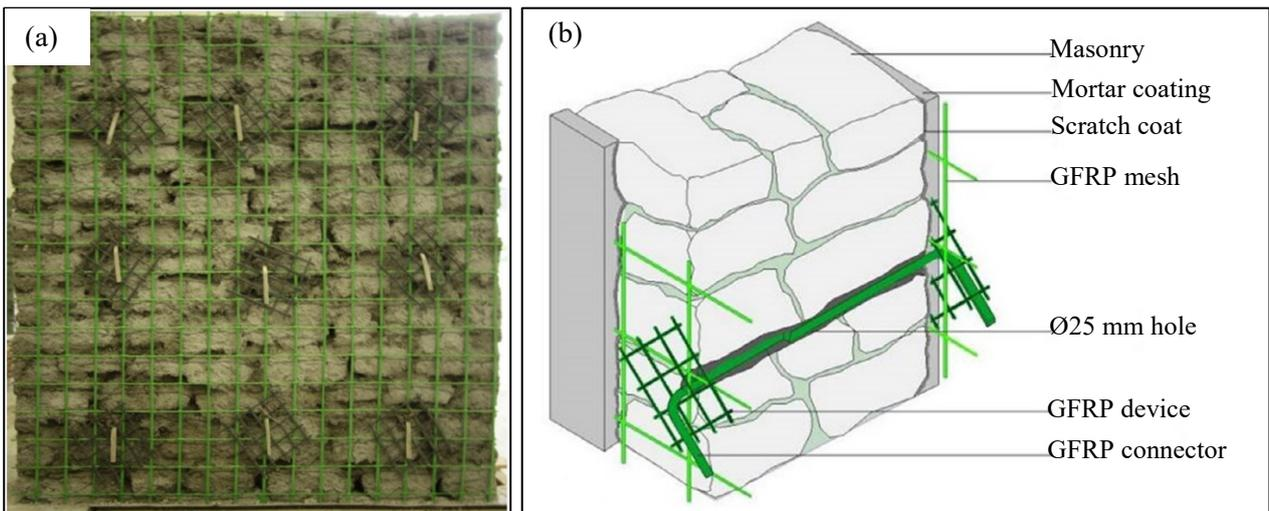
Fig. 47: GFRP mesh reinforced cementitious mortar coating on a stone wall. Application (a) and scheme(b) (Gattesco et al. 2015 & 2017)
