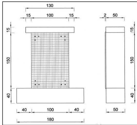
Fig. 49: Stone masonry wall strengthened only on one side by GFRP reinforced mortar coating, anchored to the wall at the corners.
