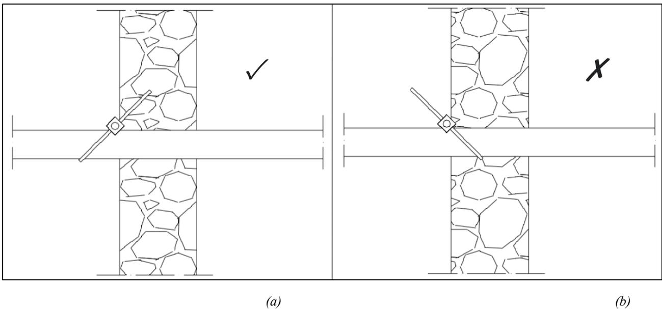
Fig. 68: Correct placing of stake anchor heads (a) and incorrect one (b).
