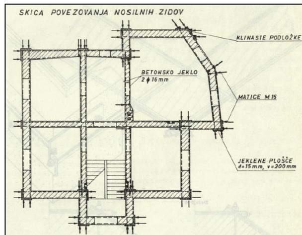
*Fig. 23: Placement of steel ties (Vugrinec, 1977)*
