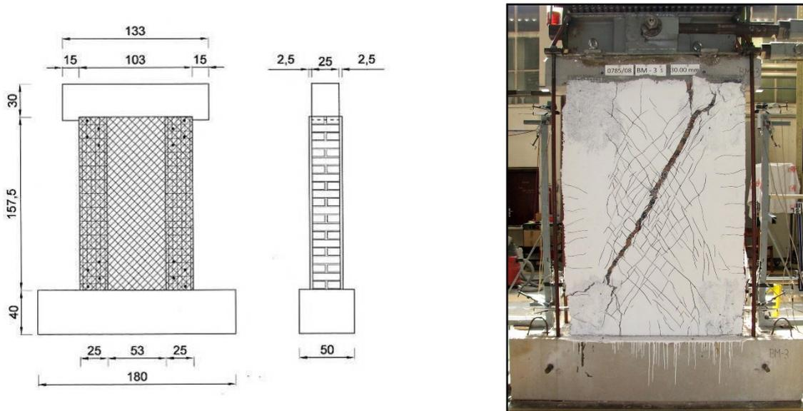
Fig. 57: GFRP layout for the wall with thickest coating, left. The failure of such wall, right.
