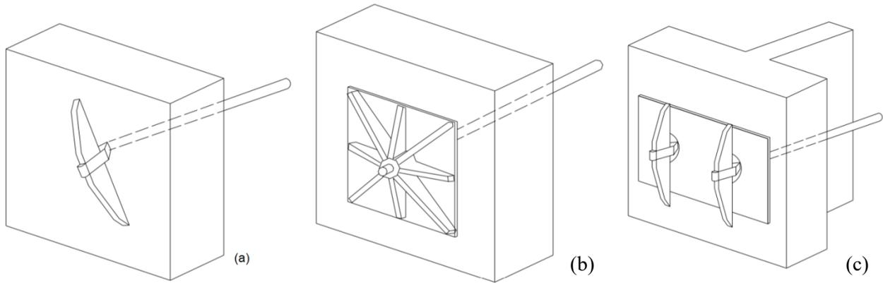
Fig. 67: Different types of anchor heads: stake type (a), ribbed plate (b), double stake and plate (c) (ReLUIS 2011)
