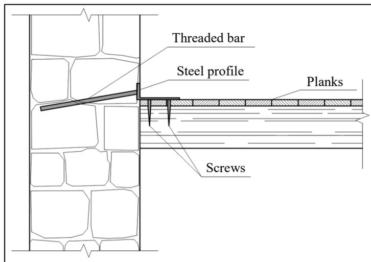
Fig. 29: Anchoring wooden floors into walls (Gattesco and Macorini, 2006; Piazza, 2008).
