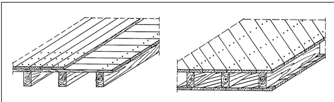
Fig. 27: Strengthening floors by an additional layer of boarding (from Tomažević, 2009)
