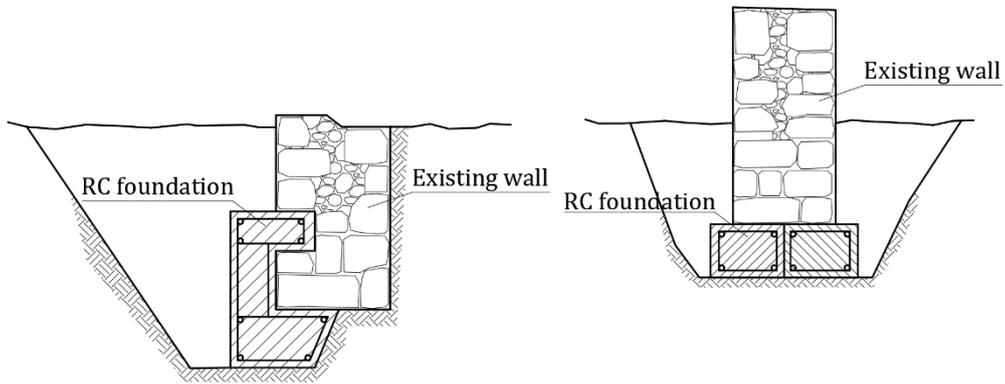
Fig. 21: Strengthening foundations by adding reinforced concrete (from Tomažević, 2009).
