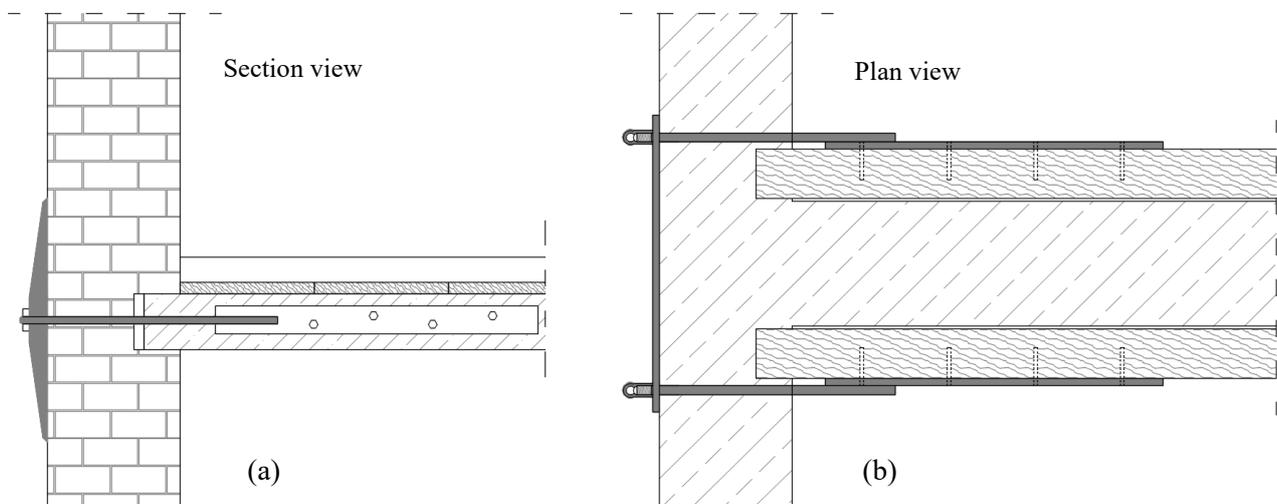
*Fig. 66: Section (a) view of a simple tie rod adherent to the transverse wall at floor level and plan view (b) of coupled tie rods adherent to the transverse wall at floor level (ReLUIIS 2011).*
