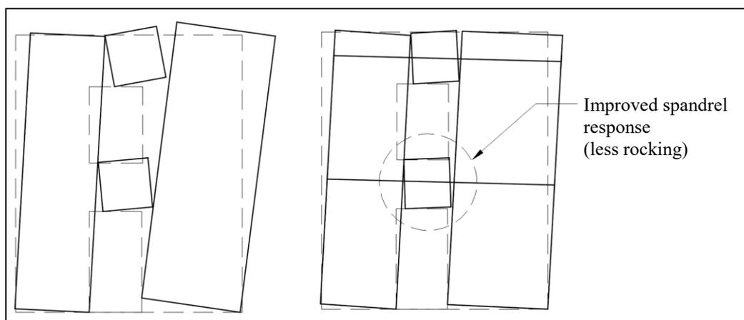
Fig. 25: Rocking of spandrels (left) is limited by ties (right).
