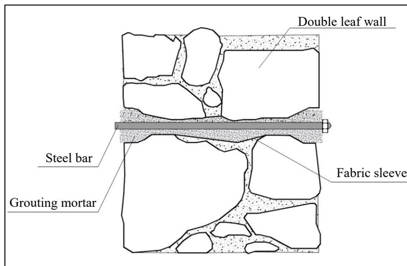
Fig. 41: Schematic view of an artificial diaton.
