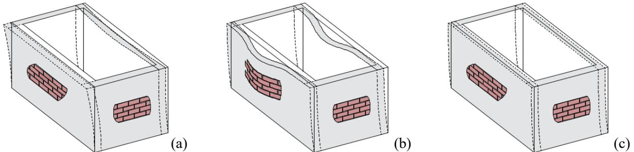
Fig. 8: Response of structures with different strength of connections: a) poor connection between walls and weak floor structure, b) proper connection between walls but weak floor structure and c) proper connection between walls and strong floor structure.
