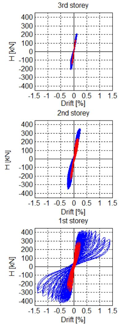
Fig. 61. Three storey pilot building before test, left. Hysteretic curves of unstrengthened (red) and strengthened (blue) structure, right
