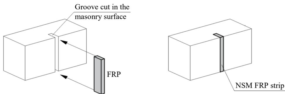
Fig. 45: Schematic representation of NSM FRP strip (Petersen, 2009).
