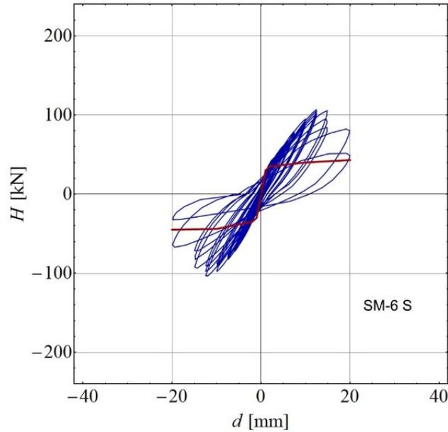
Fig. 51: Hysteretic response of stone masonry wall with one side GFRP reinforced mortar coating. Blue line shows the response of the strengthened wall and the red line indicates the resistance envelope of the reference wall.
