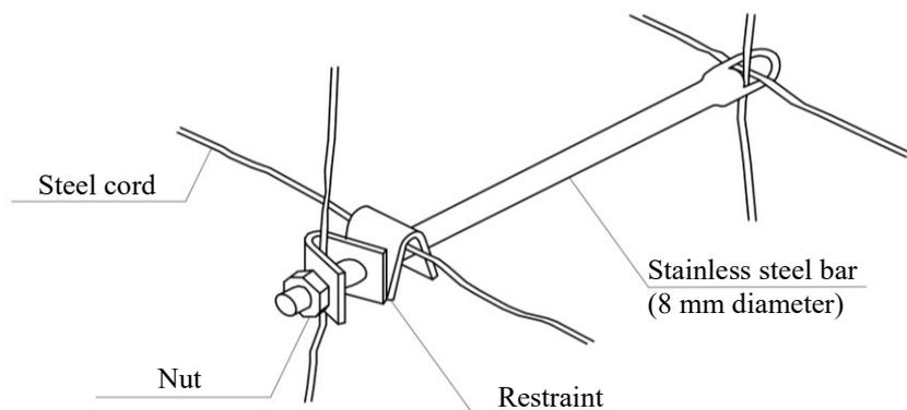
Fig. 63: Cord and eyelets disposition detail (passing through)
