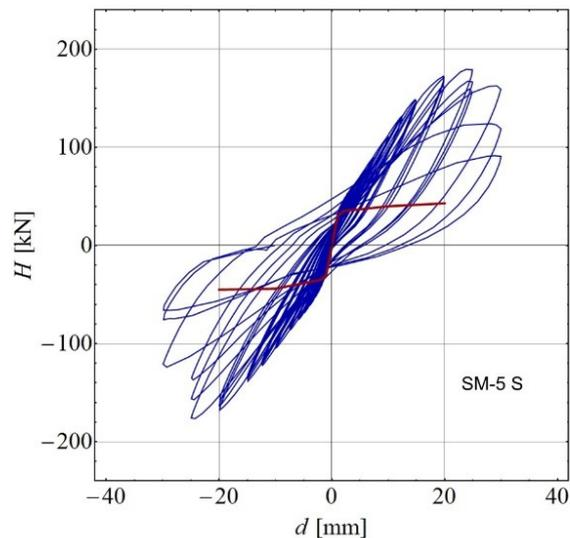
Fig. 54: Hysteretic response of stone masonry wall with GFRP reinforced mortar coating on both sides. Blue line shows the response of strengthened wall and red line indicates resistance envelope of the reference wall.
