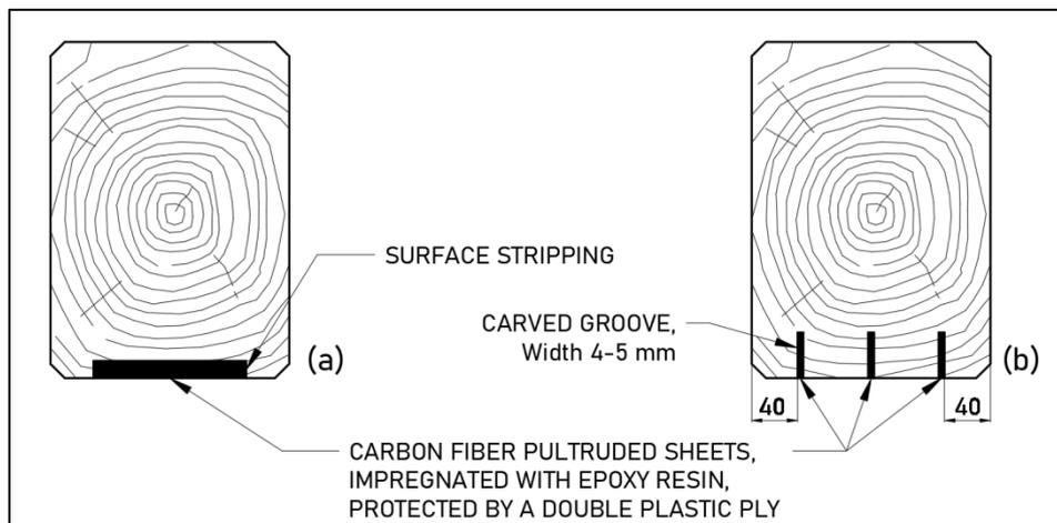
Fig. 33: Wooden beam strengthened by a single carbon fibre strip (a), and by three vertically placed strips (b).
