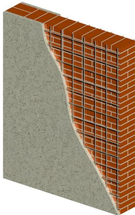
*Fig. 40: Representation of a reinforced-cement coating*
