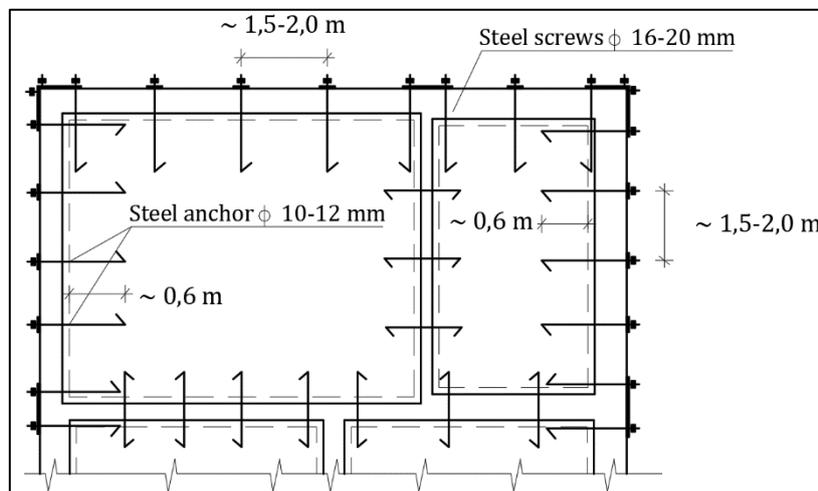
Fig. 30: Anchoring RC slab to walls by steel anchors (Tomažević, 2009).
