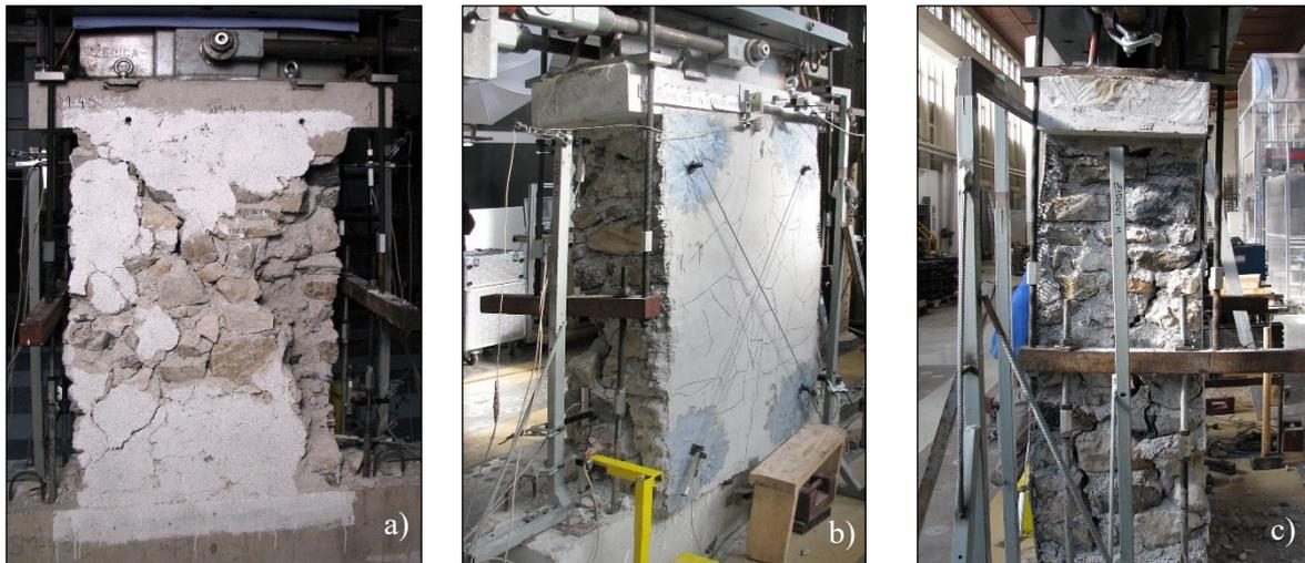
Fig. 50: Stone wall with coating on one side during test. Disintegration of the side without the coating (a), small damage on the side with the coating (b) and splitting of the wall due to lack of diatones (c).
