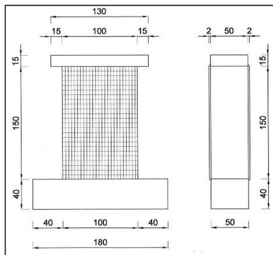
Fig. 52: Stone masonry wall strengthened by GFRP reinforced mortar coating on both sides of the wall.
