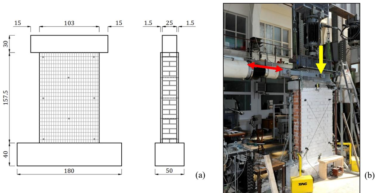
Fig. 55: Dimensions of the GFRP reinforced walls used in testing (a). Test setup for shear-compression test. Red arrow shows imposed horizontal displacements and yellow arrow shows compressive force (b).
