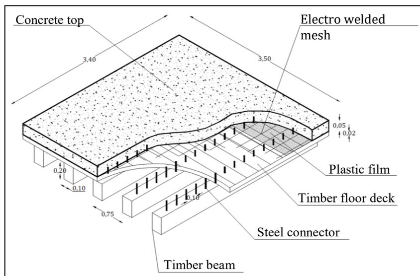
Fig. 32: Composite concrete slab - wooden floor system (Santos, 2015).
