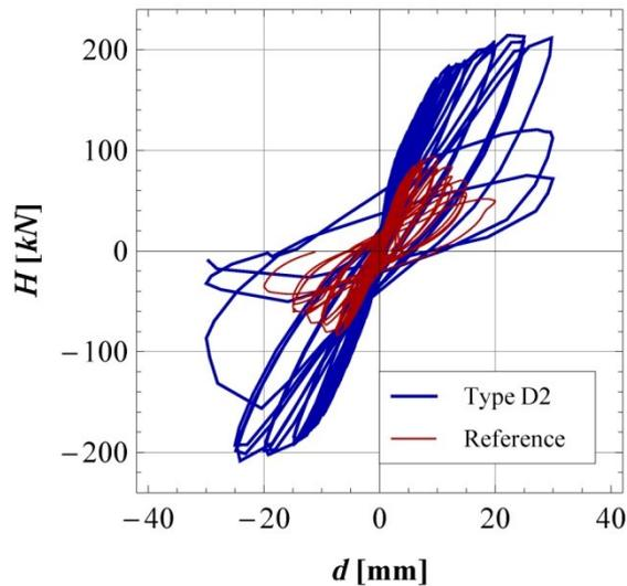
Fig. 58: Hysteretic response of brick masonry wall with 25 mm thick GFRP reinforced mortar coating on both sides and strong anchoring. Blue line shows the response of the strengthened wall and red line indicates the resistance envelope of the reference wall.
