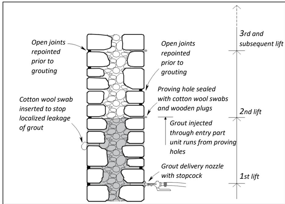
Fig. 38: The basic grouting method for filling the voids is illustrated here. (Iain McCaig, reproduced from English Heritage’s Practical Building Conservation: Stone, 2012)
