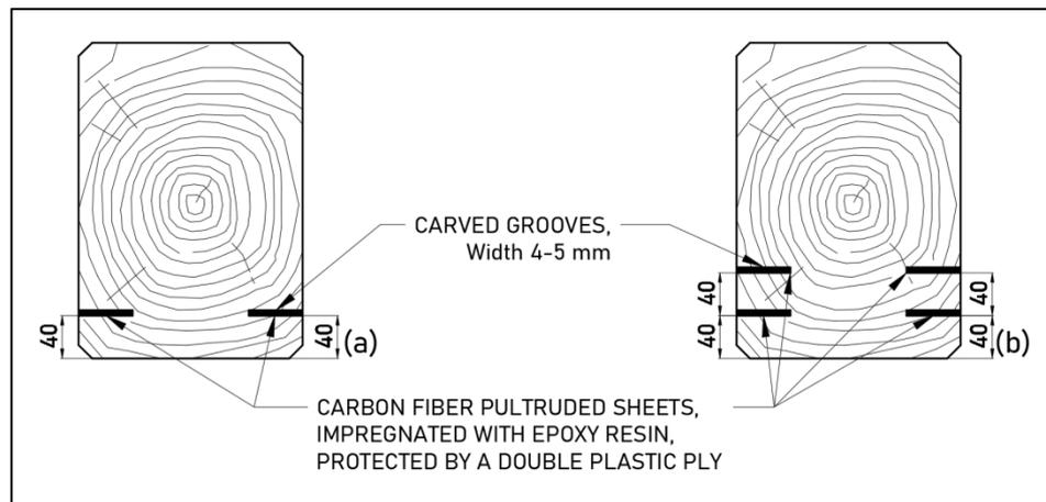
Fig. 34: Wooden beam strengthened by horizontally placed strips.
