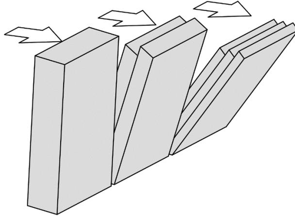
*Fig. 15: Out-of-plane behaviour of a single-leaf wall and a multi-wythe wall*
