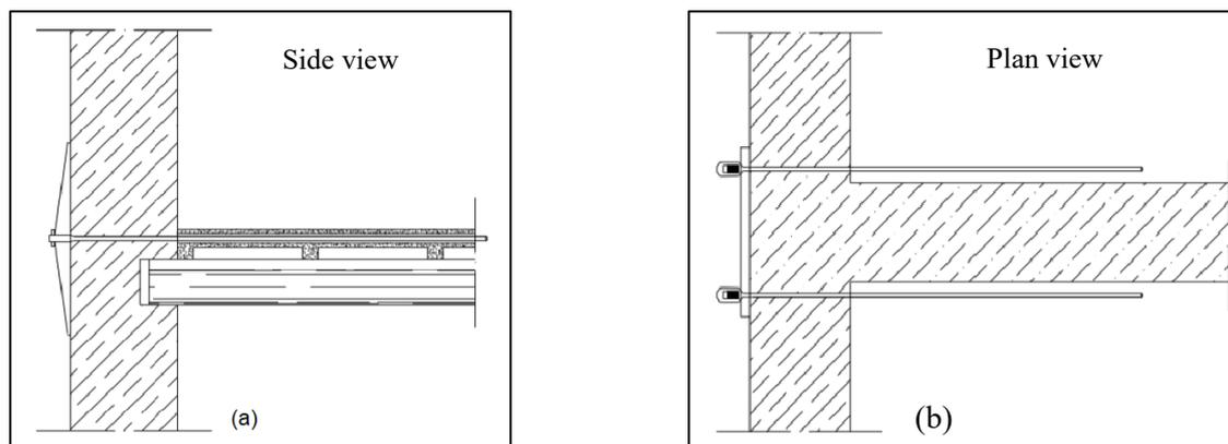
Fig. 24: Side view of a steel tie above timber joists (they are more often installed under joists) (a), and plan view of tie rods of an inner wall (b) (ReLUIS 2011)
