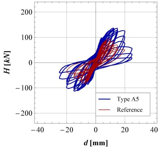
Fig. 58: Hysteretic response of brick masonry wall with GFRP reinforced mortar coating on both sides and 9 anchors/m<sup>2</sup>. The blue line shows the response of the strengthened wall and the red line indicates the resistance of the reference wall.
