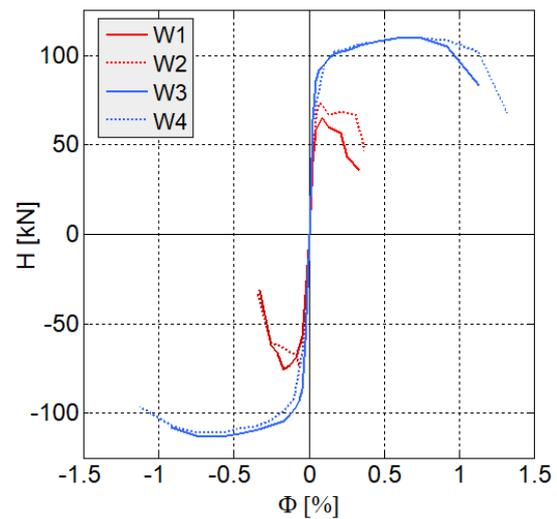
Fig. 60: Buckling of the coating, left. Envelopes of the hysteretic response of two reference walls (red) and two strengthened walls (blue), right.
