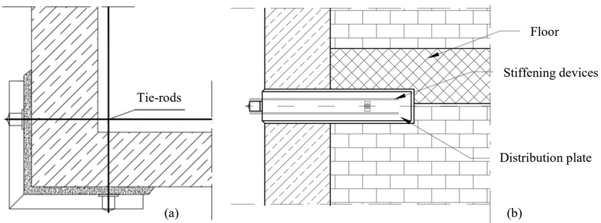
Fig. 71: Double angle tie rod: plan view (a) and perspective view (b)
