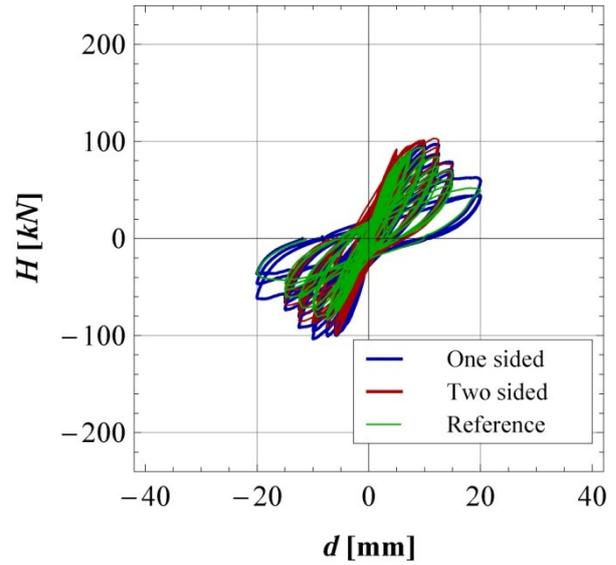
Fig. 46: Peeling off of type of debonding between coating with an epoxy matrix, left. Hysteretic response of walls with one sided and two sided GRPF reinforced coating in epoxy matrix, right (Gams et al. 2017).
