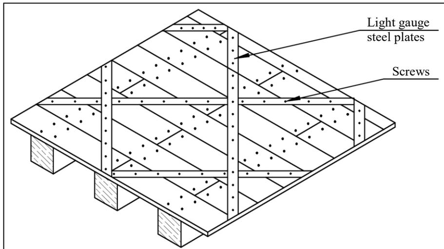
Fig. 28: Diagonal steel ties technique (Gattesco and Macorini, 2006; Piazza, 2008, Tomažević, 2009).
