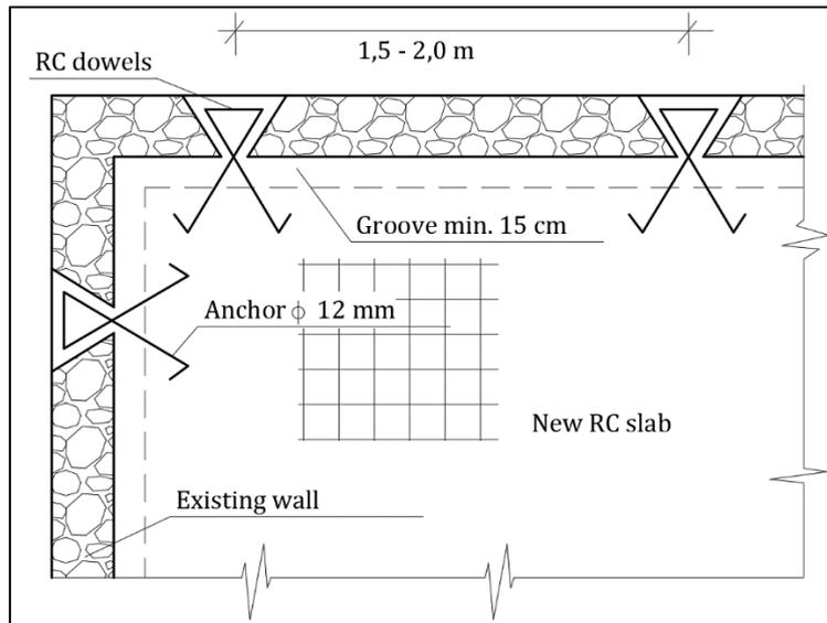
Fig. 31: Anchoring RC slab to walls by RC dowels (Tomažević, 2009).
