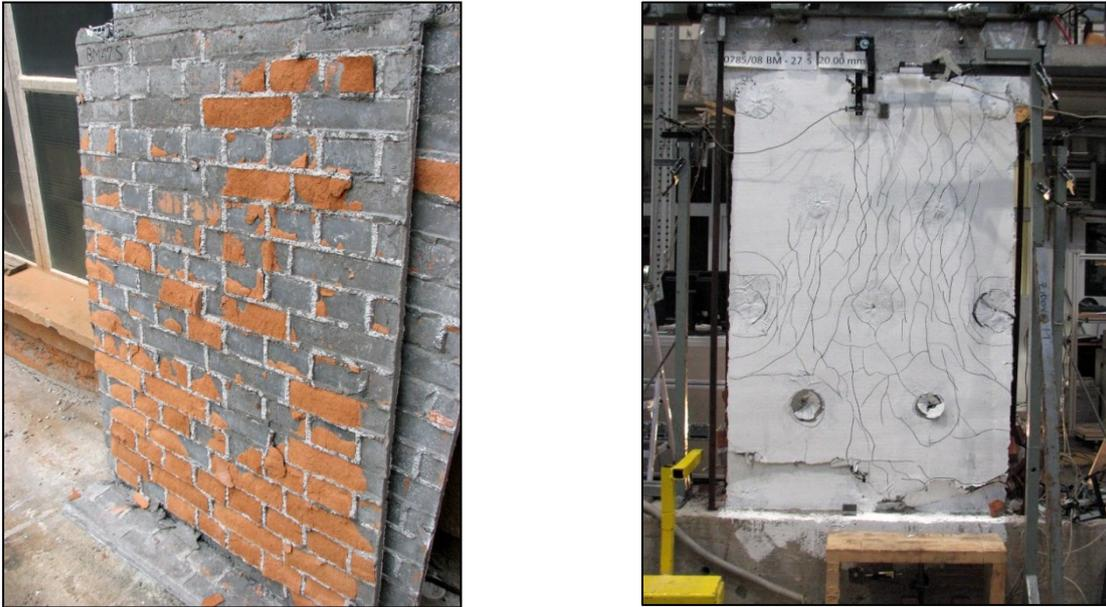
*Fig. 56: Completely separated coating without anchors (a). Failure of bond and anchors in case of highest density of anchors (b)*
