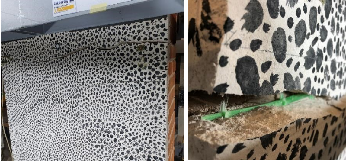
Fig. 89: Fracture of GFRP mesh at collapse.
