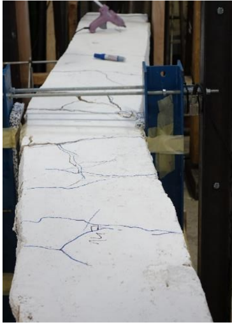
Fig. 143: Side view of T-R2 at collapse.
