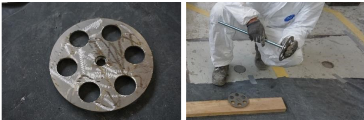
Fig. 8: Steel connector or "artificial diaton".
