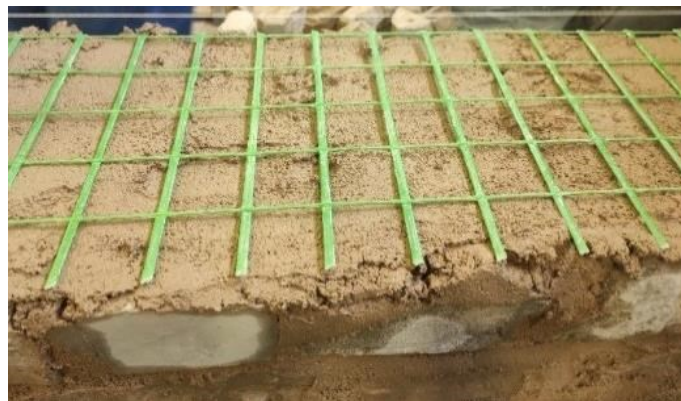
Fig. 141: Mesh embedded in the bed joint.
