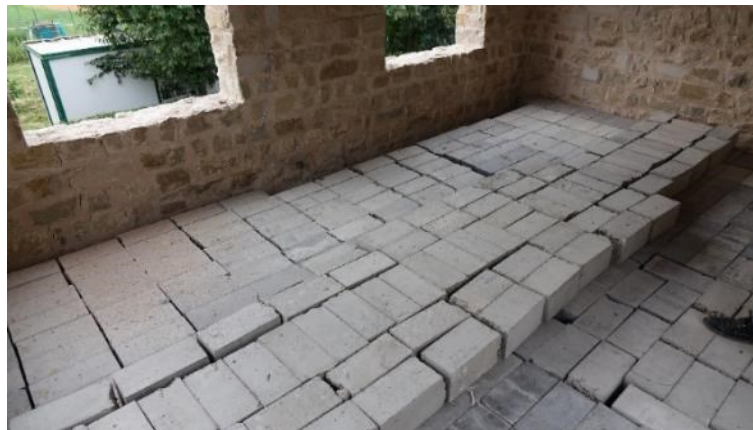
Fig. 176: Concrete block weights for simulation of the load in the structure
