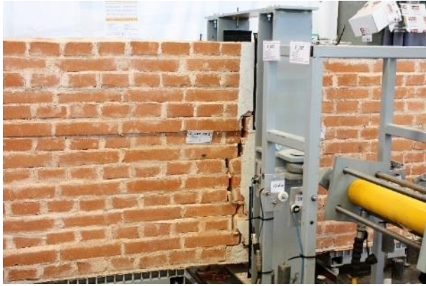
Fig. 166: crack configuration during the monotonic test – flexural cracks at step 12 (-40.6 mm)
