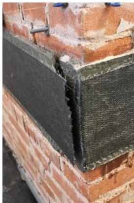
Fig. 167: failure of the CFRP strip in the right corner at -50.4 mm
