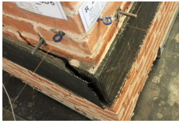
Fig. 167: failure of the CFRP strip in the right corner at -50.4 mm
