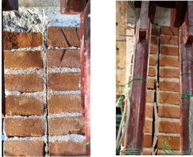
Fig. 52: (P-B2U) Separation of wall leaves at 8 mm (left) and 15 mm (right)
