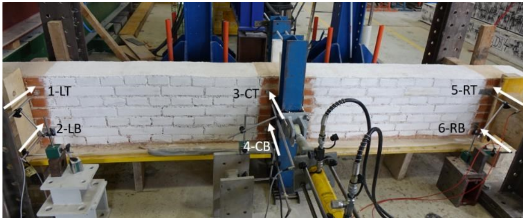
Fig. 139: Locations of displacement transducers.
