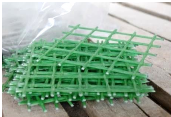
Fig. 6: Mesh sheets with smaller spacing to use with L connectors.
