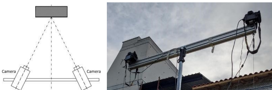
Fig. 25: The concept of locating a point in 3D using two cameras, left. The cameras used in the project, right.
