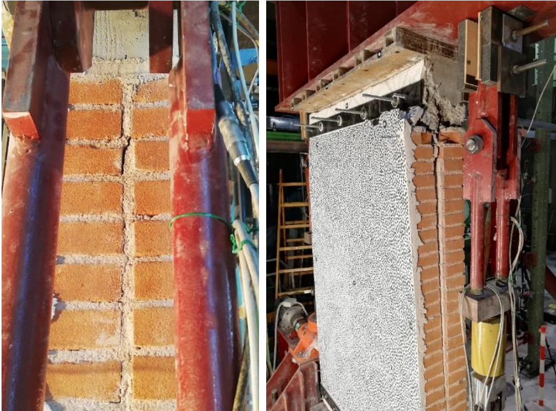
Fig. 56: (P-B2R-1) Vertical crack between wall leaves at 10 mm (left) and separation of leaves at 70 mm (right).
