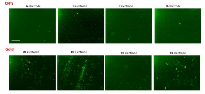
**Fig.2:** Fluorescence images of antibody bound on CNTs electrode and gold electrode acquired with a 40x objective; FITC filter. Bar 50 μm.
