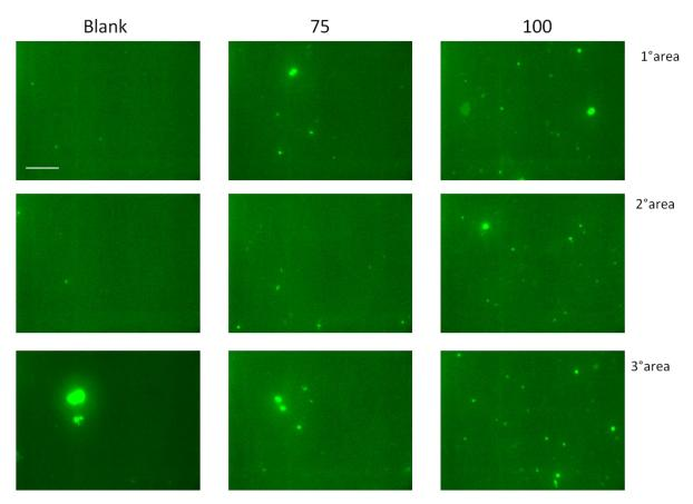
**Fig.1:** Fluorescence images of specific antibody bound on CNTs electrode acquired with a 40x objective; FITC filter. Blank is bare CNTs in absence of antibody, 75 and 100 are different concentration of antibody. Images were acquired on 3 different areas for each samples (Bar 50  $\mu$ m)
