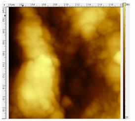
**Fig.4:** Contact mode AFM images of bare gold electrode and self-assembled monolayer of on gold electrode (cantilever Bruker MLCT K=0.02N/m).
