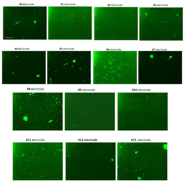
**Fig.3:** Fluorescence images of specific antibody bound to SAM functionalized gold electrodes acquired for several electrodes, 40x objective and FITC filter (Bar 50 μm).
