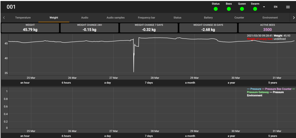
Picture 6: The mass of the hive being weighed.
