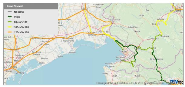
Figure 4 – Thematic representation of allowed speed in the TEN-T railway links. Source: TENtec
